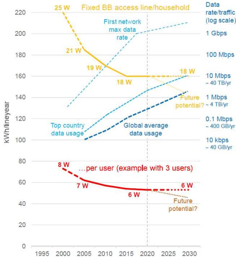
**Figure 33: Average power, electricity use and data per fixed BB line (Malmö 2020)**
