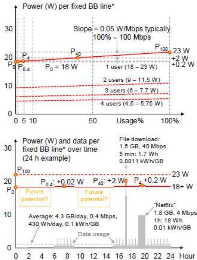
**Figure 31: Power/data and power/time (24 h) model for a fixed BB access line (household)<sup>19</sup> (Malmodin 2020)**
