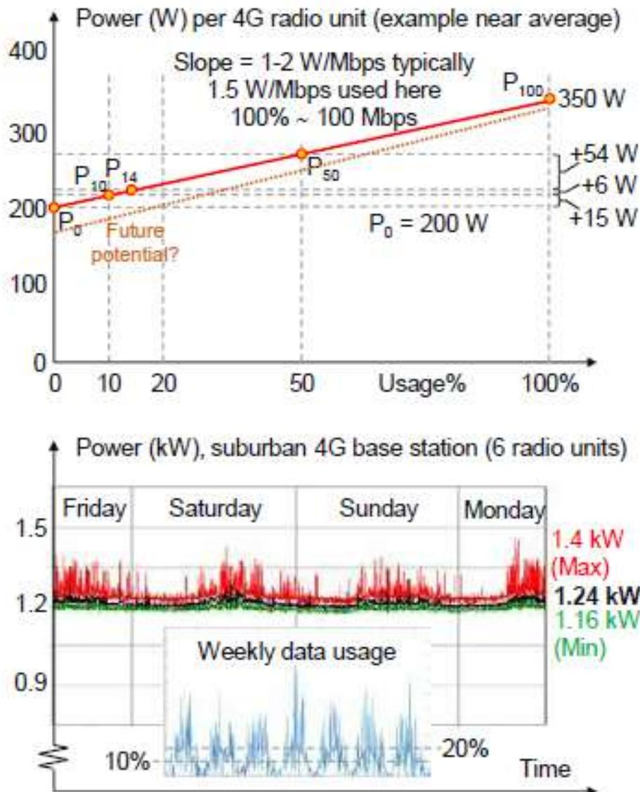
**Figure 30: Power and data model for suburban 4G radio unit / base station (based on real data) (Malmudin 2020)**
