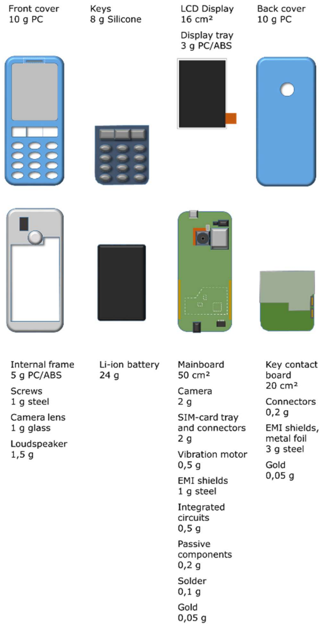
Figure 23 : Feature phones – major parts, materials and weights
