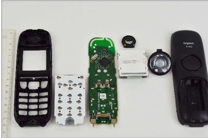
Figure 48 : Cordless phone handset teardown – frontside cover inside view, key pad backside, mainboard reverse side, display unit backside view, loudspeaker, backside cover
