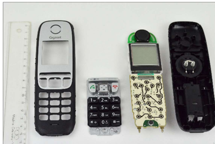
Figure 47 : Cordless phone handset teardown – frontside cover, key pad, display and mainboard, backside cover
