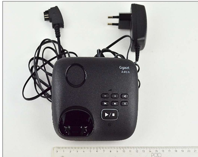
Figure 50 : Cordless phone base station teardown – overview
